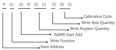
③Instantaneous and Accumulated flow rate value to zero synchronously
