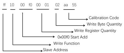
②Accumulated flow rate value to zero
