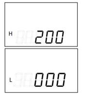
①View the maximum alarm value for the set instantaneous flow rate (stable display H \*\*\*, H 200 is the default upper limit);
