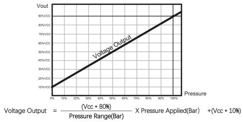
Figure 1 Voltage output curve and formula
