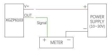
Figure 6 Application Circuit (Current Output)
