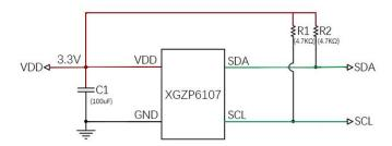
Figure 7 Application Circuit (I2C Interface)
