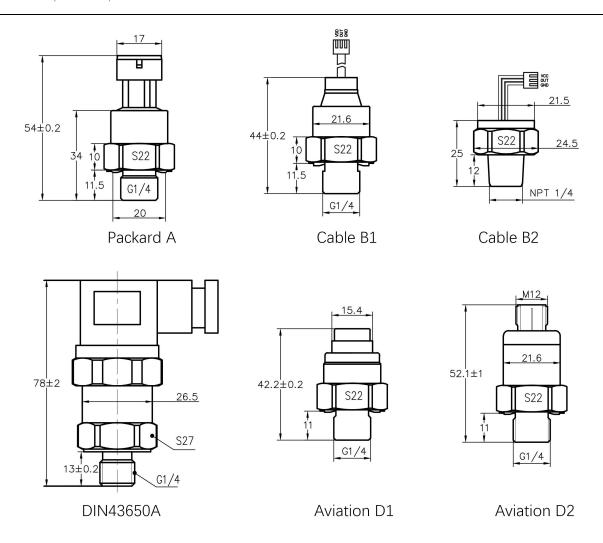
Figure 4 Structure Dimension
