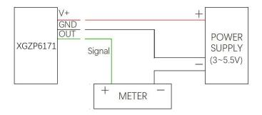
Figure 5 Application Circuit (Voltage Output)
