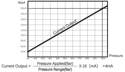
Figure 2 Current output curve and formula
