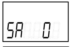
①Check the set switching value (normal display **SA** \*): '\*' bit shows '0' for 4-20mA output, display '1' for 0-5V/10V output;
