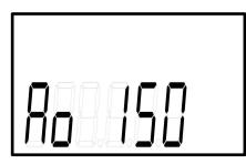
④ Check set current 4-20mA lower current 4mA calibration value (normal display A0 \*\*\*, default 120) ;
